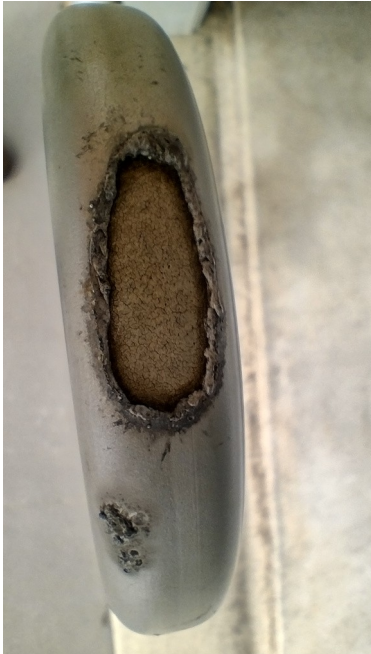
Left image shows the top of the old antenna is burnt through from a lightning hit. Right image shows where the boom for the aerial clamped onto the mast and it also arced on the high resistance joint of this boom to mast clamp.
