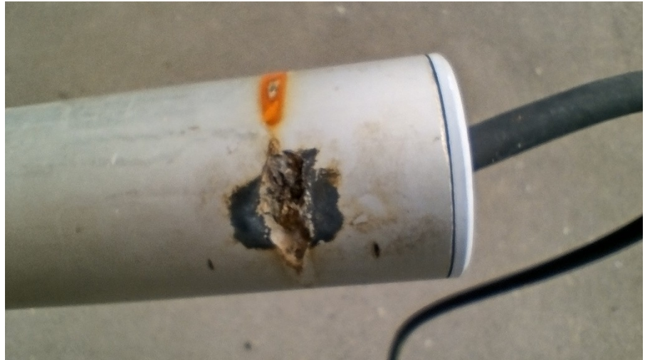
Left image shows the top of the old antenna is burnt through from a lightning hit. Right image shows where the boom for the aerial clamped onto the mast and it also arced on the high resistance joint of this boom to mast clamp.
